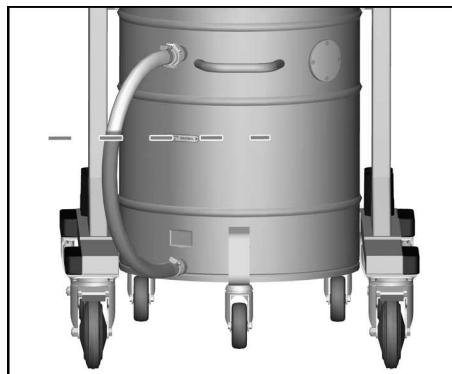
**Note:** The red marking on the drain hose shows the maximum admissible filling level.
