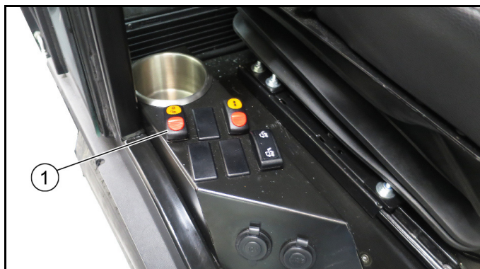
① Battery disconnecter relay
