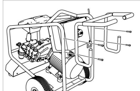
Fasten the pushing handle with the four screws enclosed in the packet.
