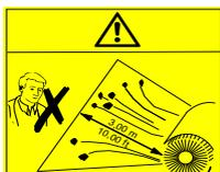
Hazard caused by ejected parts with moving roller brush. Keep a safety distance of 3 m towards the front and the side
