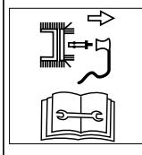
Switch the machine off prior to any work, such as adjustments, cleaning, testing and pull the spark plug.
