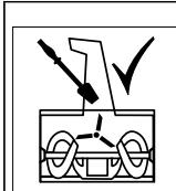
Only clean the discharge chute with cleaning utensils..
