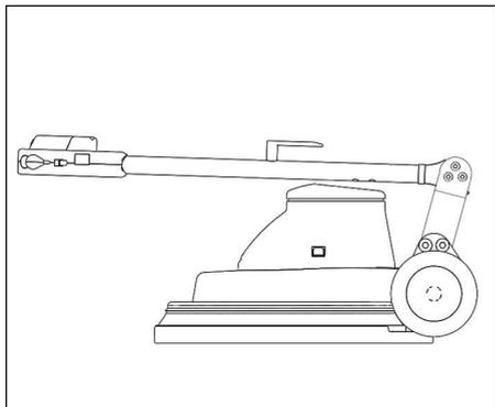
With the 230V/60Hz variant the handle can be swivelled to the front for transport and storage.
