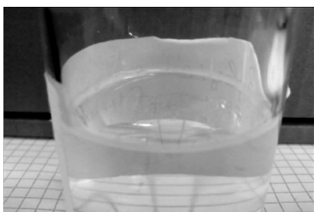
Foam picture filter OK: very thin foam ring on the edge, which disintegrates quickly.
