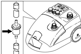
Using soiled water can occlude the filter. This is shown by extraordinarily long run times of the pump or a complete malfunction.
