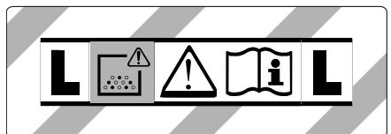
**WARNING:** This appliance contains harmful dust. The emptying and maintenance, including the removal of the dust bag, may only be executed by trained personnel wearing suitable protection equipment. Do not switch on until the complete filter system has been installed.
